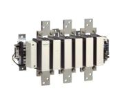
contactor body withou coil, TeSys F, 3P(3NO), AC-3, <=440V 780A,use with coil LX1/LX9 110…500V AC 40/400Hz, LX4 110...440V DC
